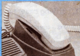
Specially designed "universal" cradle accepts all types of handsets. Unit is automatically switched on when handset is placed on cradle.
