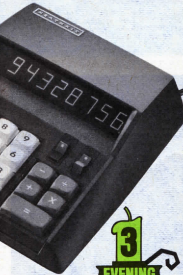
Components mount on one roomy circuit board, and there's an internal adjustment to compensate for high or low line voltage.
