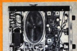
Modular circuit-board design simplifies assembly.
