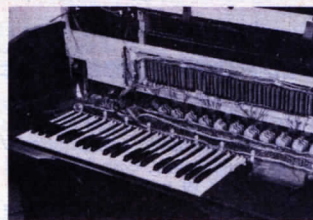
Manual boards lift for easy access to circuitry
