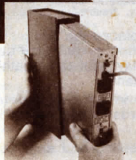
The simulated book cover leaves rear panel exposed for easy access to switches and plug outlets. Unit can be used without cover if desired.
