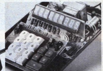
Components mount on one roomy circuit board, and there's an internal adjustment to compensate for high or low line voltage.
