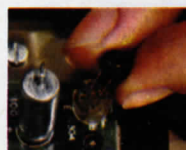
Socket-mounted transistors & ICs.
