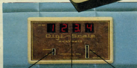
Manual or auto turn-on Bright red 4-digit LED display Handy zeroing adjustment
