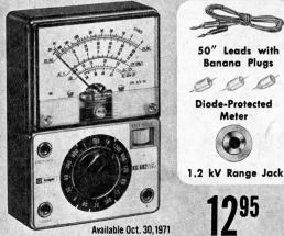
Knight-Kit KG-682. The ultimate in VOM portability! 1% tolerance resistors used as multipliers give extra accuracy, stability. Zero-adjust assures accurate calibrations—compensates for changes in battery condition. Easy-to-read scale. Complete with 50" leads, banana plugs, battery.  $3^1\%_6 \times 5^1/_2 \times$
